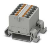
Distribution block, Block with horizontal alignment, nom. voltage: 800 V, nominal current: 32 A, connection method: Push-in connection, number of connections: 12, cross section:0.2 mm² - 6 mm², AWG: 24 - 10, width: 36.9 mm, color: gray, mounting type: NS 35/7,5, NS 35/15
