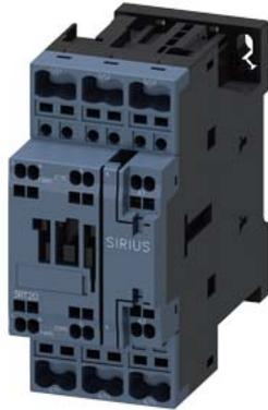
power contactor, AC-3 25 A, 11 kW / 400 V 1 NO + 1 NC, 480 V AC, 60 Hz
