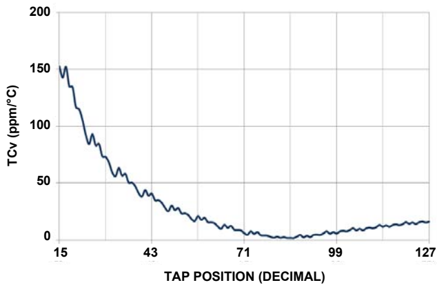
FIGURE 13. 10kΩ TCv vs TAP POSITION, V_{CC} = 3.3V
