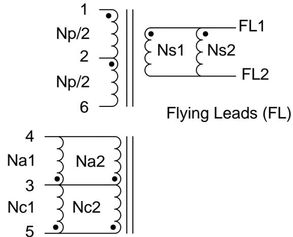
Figure 22. Transformer Schematic
