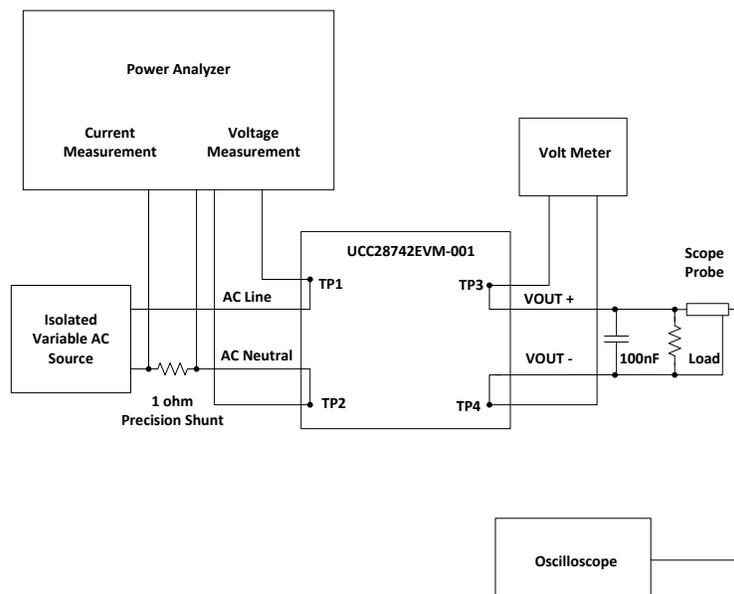
**Figure 3. UCC28742EVM-001 Test Setup Diagram**
