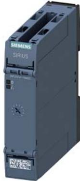
Timing relay, electronic with star-delta (wye-delta) function 1 NO delayed 1 NO instantaneous 1 time range, 1...20 s 200-240 V AC and 380-440 V AC screw terminal
