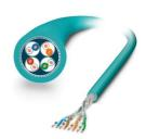
Data cable, Ethernet  $CAT6_A$  (10 Gbps), 8-position, PUR halogen-free, water blue RAL 5021, shielded, free cable end, on free cable end, cable length: 300 m
