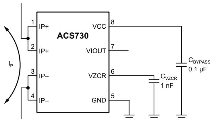
The ACS730 outputs an analog signal,  $V_{IOOUT}$ , that varies linearly with the bidirectional AC or DC primary sensed current,  $I_p$ , within the range specified.
