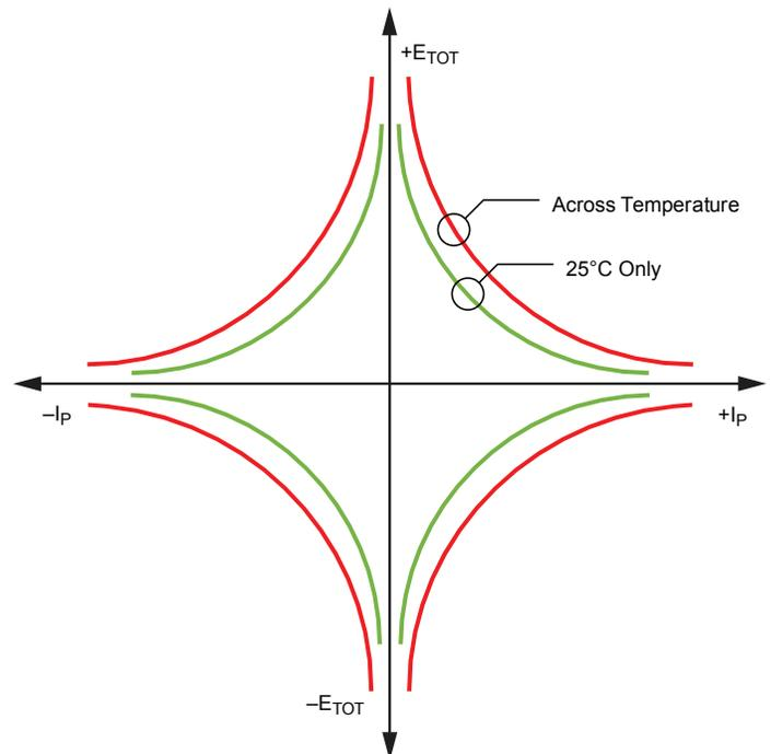
Figure 2: Total Output Error versus Sensed Current
