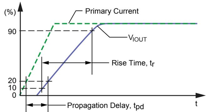
Figure 4: Rise Time ( $t_r$ ) and Propagation Delay ( $t_{pd}$ )
