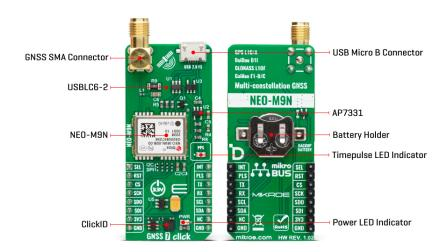
Note: Button battery 1.55V is provided with the GNSS 7 click
