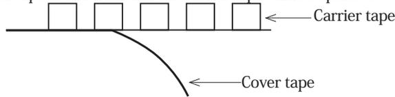
**(3) Taping method and marking**
