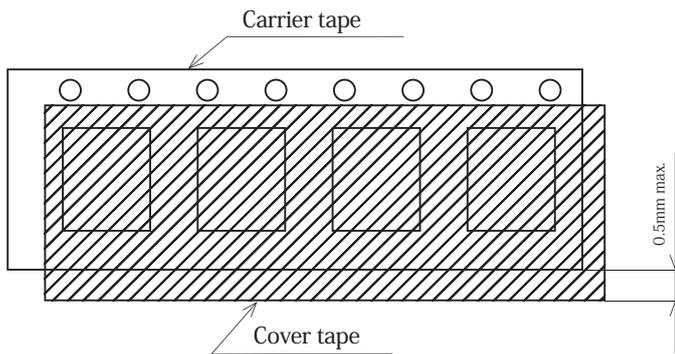
The cover tape shall not extend exceeding 0.75mm to the sprocket holes.
