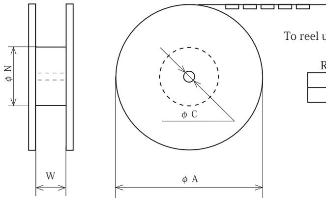
To reel up the tape so that the parts can face the reel core.
