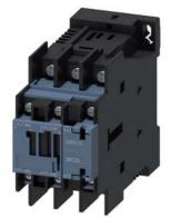
power contactor, AC-3 25 A, 11 kW / 400 V 1 NO + 1 NC, 24 V DC 3-pole, Size S0 ring cable lug connection
