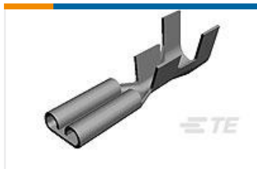
TE Part #41969-2 250 FASTON REC 22-18 AWG BR
