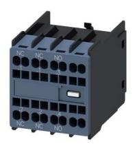
Auxiliary switch on the front, 1 NO + 2 NC Current path 1 NC, 1 NO, 1 NO for 3RH and 3RT spring-type terminal .1/.2, .1/.2, .3/.4
