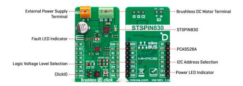
To control all high and low side driver control inputs of the STSPIN830, Brushless 13 Click features the <u>PCA9538A</u>, a low-voltage 8-bit I2C I/O port with interrupt and reset from NXP. Besides driver control inputs, this I/O port also controls the enable input of the motor driver. The BLDC motor can be connected over the screw terminal, labeled U, V, and W. Additional screw terminal is just aside for connecting an external power supply in a range of 7V up to 45V.
