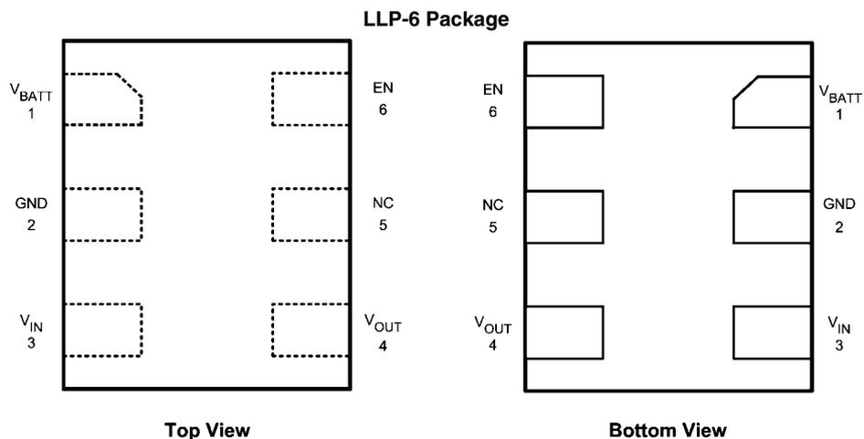
**Connection Diagram 6-Pin Chip On Lead LLP package, 0.5mm pitch**
