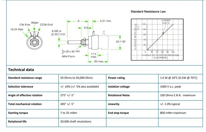
General purpose wirewound panel control of robust and reliable construction. Phenolic body moulding; beryllium copper contact; nickel plated brass spindle and bush; silver plated brass tags
