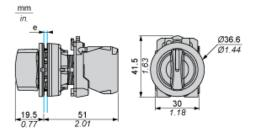
: Clamping thickness: 1 to 6 mm / 0.04 to 0.24 in.
