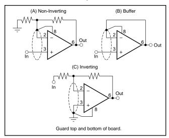
FIGURE 2. Connection of Input Guard.
