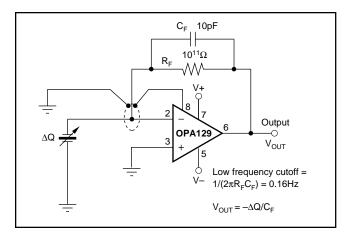
FIGURE 6. Piezoelectric Transducer Charge Amplifier.
