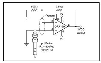
FIGURE 5. High Impedance ( $10^{15}\Omega$ ) Amplifier.
