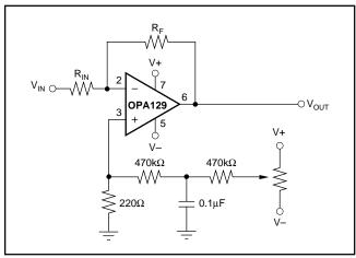
FIGURE 1. Offset Adjust Circuit.
