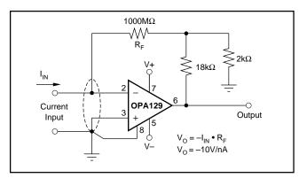
FIGURE 4. Current-to-Voltage Converter.
