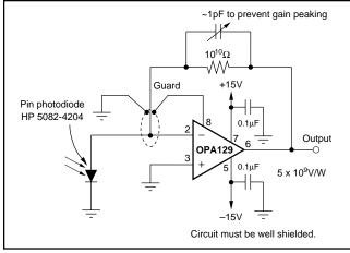
FIGURE 7. Sensitive Photodiode Amplifier.
