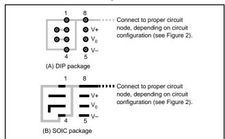
FIGURE 3. Suggested Board Layout for Input Guard.
