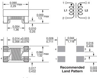
Dimensions are in  $\frac{\text{inches}}{\text{mm}}$
