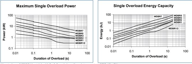
Mounted on a 0.53°C/W heatsink with 5m/s forced air cooling, air temperature 25°C.  $\Delta R \le 5\%$ .
