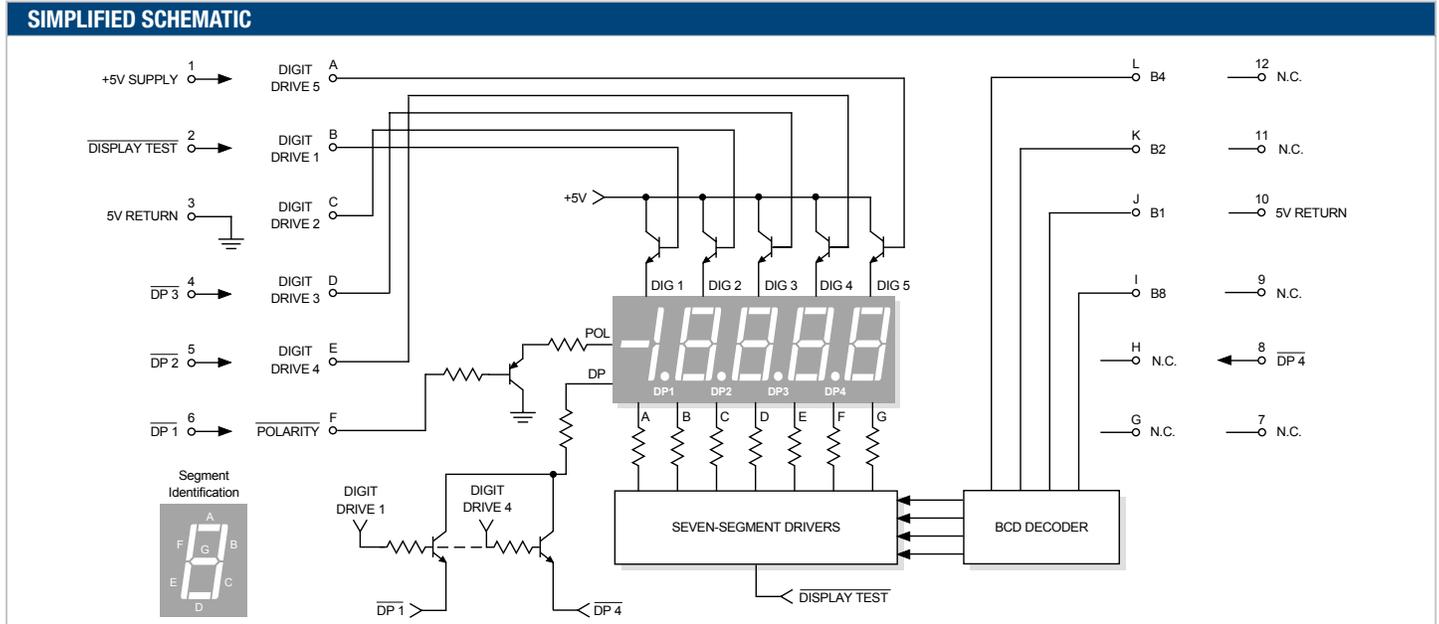
Figure 1. Simplified Schematic
