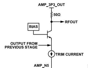
Figure 4. AD9166 Equivalent Output Circuit for RFOUT
