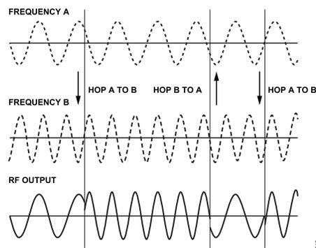
Figure 8. Diagram of Phase Coherent Frequency Hopping
