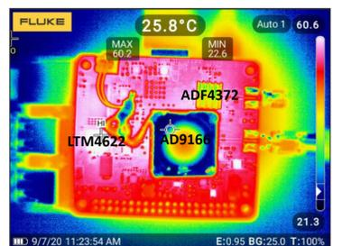
Figure 14. CN0511 Thermal Performance with Heat Sinks Attached
