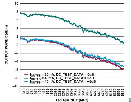
Figure 5. AD9166 Uncalibrated Output Power vs. Frequency
