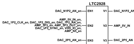
Figure 12. CN0511 Power Sequencing Simplified Diagram
