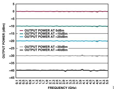
Figure 6. CN0511 Calibrated Output Power vs. Frequency
