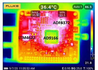
Figure 13. CN0511 Thermal Performance without Heat Sinks Attached
