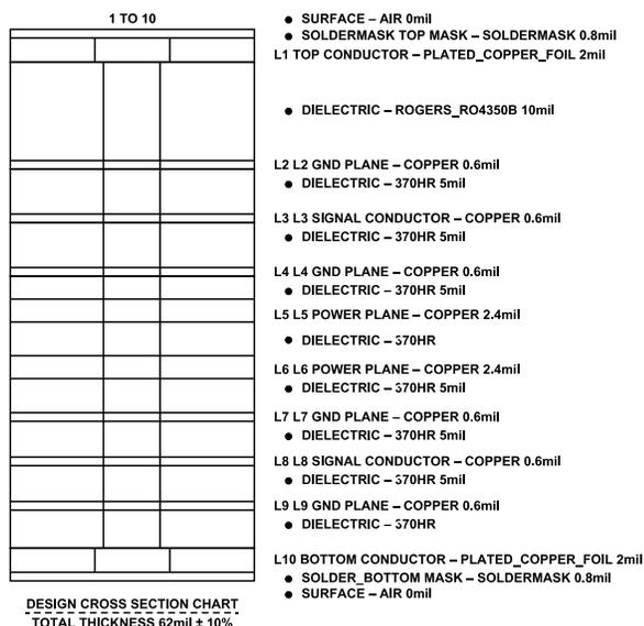
Figure 15. CN0511 PCB Cross Section and Stackup
