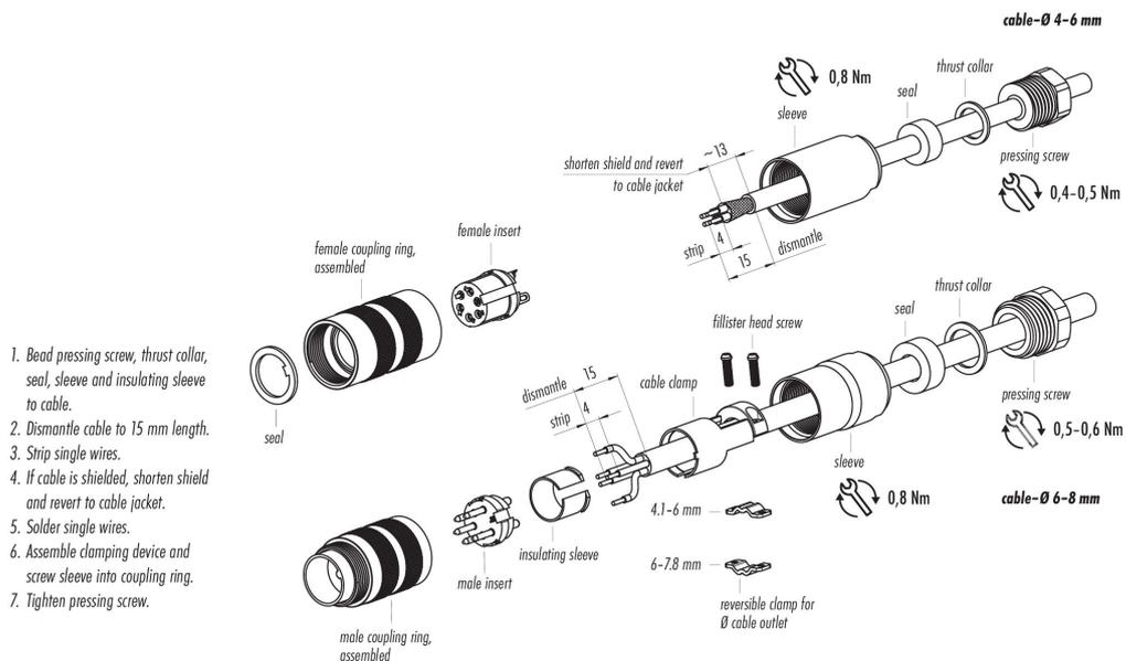
1. Bead pressing screw, thrust collar, seal, sleeve and insulating sleeve to cable.
