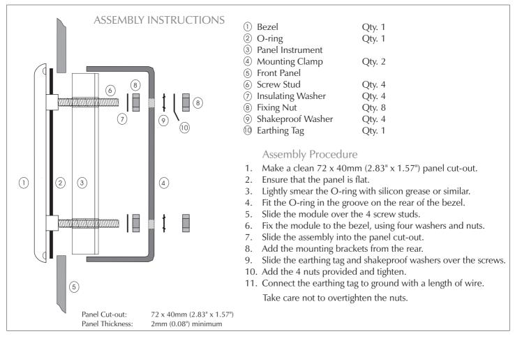
Notes: On some panel instruments it may be easier to configure links and calibrate the product prior to fitting the instrument and BEZ 900-IP into the panel. Always observe safety warnings on the Panel Instrument datasheet.
