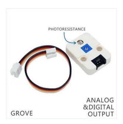
A photoresistor is a light-controlled variable resistor. The resistance of a photoresistor decreases with increasing incident light intensity, and vice versa. It exhibits photoconductivity which make it possiable to detect the varies based on Voltage, and use a AD to convert the digital data.
