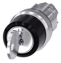
RONIS key-operated switch, 22 mm, round, metal, shiny, lock number SB30, with 2 keys, 3 switch positions I-O<II, left latching, right momentary contact type, actuating angle  $2x45^{\circ}$ , 10:30h/12h/13:30h, key removal O, possible special locks: SB31, 421, 455
