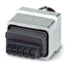
Power connector, degree of protection: IP65, number of positions: 5, material: Zinc die-cast, connection method: Spring-cage connection, connection cross section: AWG 18- 13, cable outlet: straight, color: silver
