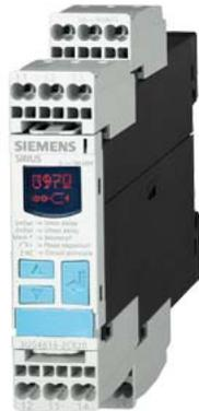
Digital monitoring relay for 3-phase voltage with N-conductor Phase sequence can be activated Phase failure 3 x 90 to 400 V 50 to 60 Hz AC Undervoltage and overvoltage 90-400 V Hysteresis 1-20 V 0-20 s each for Umin and Umax 1 CO for Umin 1 CO for Umax Spring-type terminal
