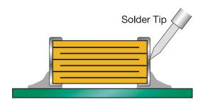
Poor Method - Direct Contact with Part
