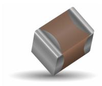
High value, low leakage and small size are difficult parameters to obtain in capacitors for high voltage systems. KYOCERA AVX special high voltage MLC chip capacitors meet these performance characteristics and are designed for applications such as snubbers in high frequency power converters, resonators in SMPS, and high voltage coupling/dc blocking. These high voltage chip designs exhibit low ESRs at high frequencies.
