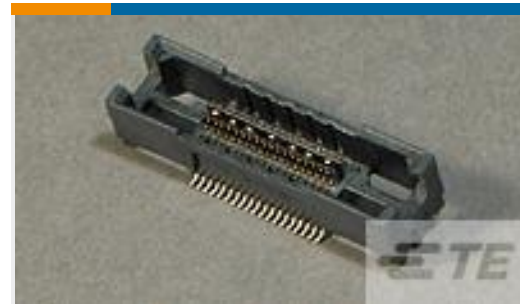
TE Part #5767171-1 MICTOR RECEPT ASSY, 38 POS. TA
