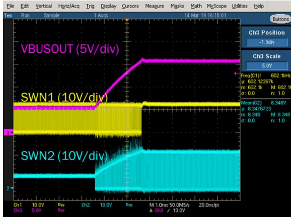
Figure 12 - 5V to 15V transition with no load
