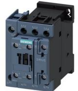
contactor AC-1, 50 A, 400 V / 40 °C, 4-pole, 110 V AC, 50 Hz / 120 V, 60 Hz, auxiliary contacts: 1 NO + 1 NC, screw terminal, size: S0
