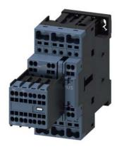
power contactor, AC-3 12 A, 5.5 kW / 400 V 2 NO + 2 NC, 110 V AC, 50 Hz 3-pole, Size S0 Spring-type terminal Removable auxiliary switch
