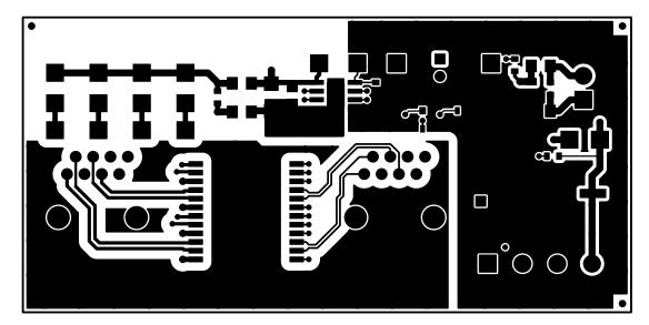
Figure 4. Top Side Routing
