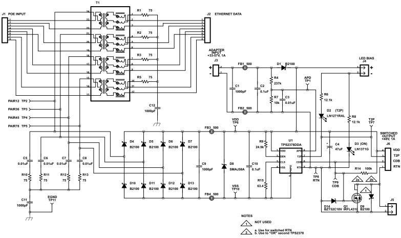
Figure 1. TPS2378EVM Schematic
