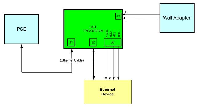
Figure 2. Typical TPS2378EVM Test Setup
