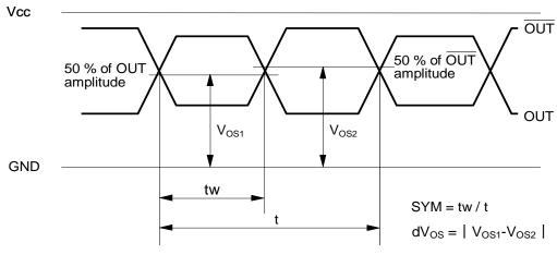
Differential output waveform (OUT –  $\overline{OUT}$ )
