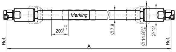
All dimensions are in mm; tolerances: ± 3mm for A ≤ 300 mm; ± 1% for A > 300 mm
