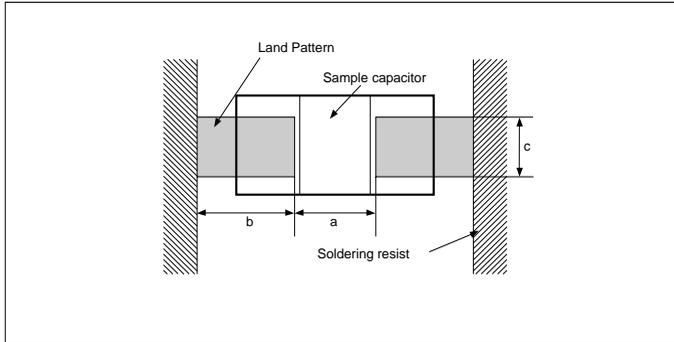
When mounting the capacitor to the substrate, it is important to consider carefully that the amount of solder (size of fillet) used has a direct effect upon the capacitor once it is mounted.
