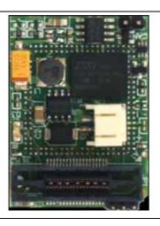
SPC563MxxAVBx Vertical base board for SPC563x line and moreover the board enables the use of new enhanced automotive calibration and debug tools on the SPC563Mx line of automotive microcontrollers, featuring a 16-bit bus interface.
