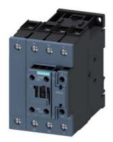
power contactor, AC-3, 35 A, 18.5 kW / 400 V, 4-pole, 24 V AC, 50 Hz, main contacts: 2 NO + 2 NC, auxiliary contacts: 1 NO + 1 NC, screw terminal, size: S2
