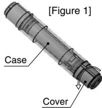
3. Pull the cover out of the case to remove the element. Remove dust and other debris remaining inside the case by blowing it out with air, etc. (Also, confirm that the O-ring is not damaged.)
