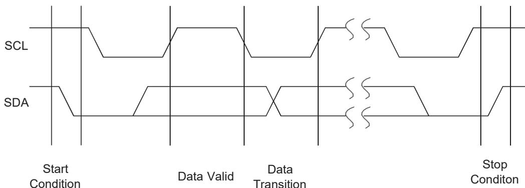
Figure2: Timing diagram for output ACKNOWLEDGE
