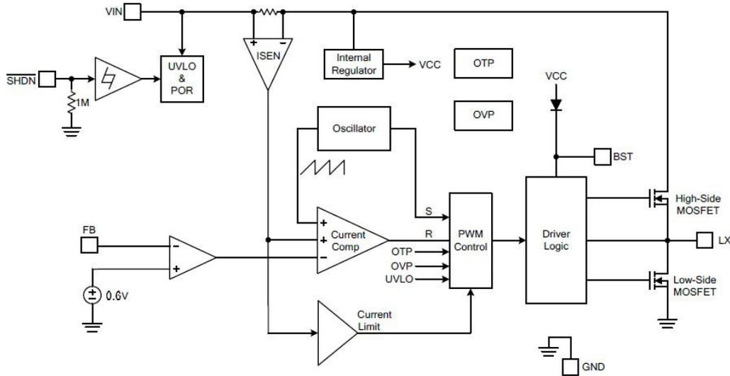
Figure 2. TMI3280 Block Diagram
