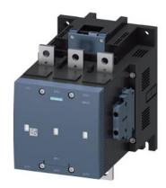
Vacuum contactor, AC-3 500 A, 250 kW / 400 V AC (50-60 Hz) / DC operation 21-27.3 V UC Auxiliary contacts 2 NO + 2 NC 3-pole, Size S12 Busbar connections Drive: electronic with PLC interface 24 V DC
