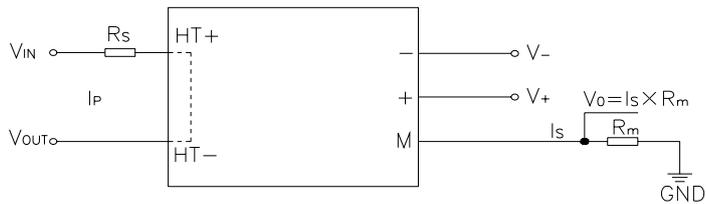
$$I_P = (V_{IN} - V_{OUT}) / (R_S + 630) \text{ BST2-5IOV2MA}$$
