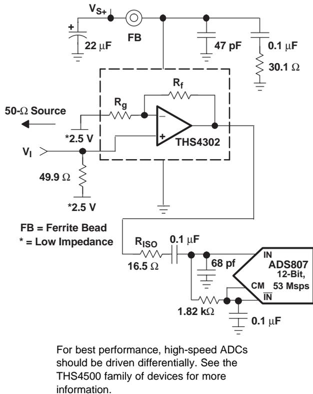
Figure 47. Driving an ADC With a Single-Ended Input
