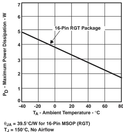
**Figure 51. Maximum Power Dissipation vs Ambient Temperature**
