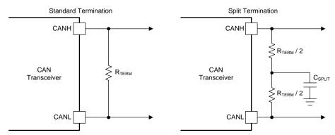
Figure 31. CAN Bus Termination Concepts
