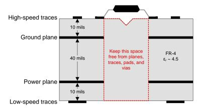
Figure 33. Recommended Layer Stack
