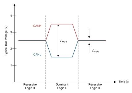
Figure 25. Bus States (Physical Bit Representation)
