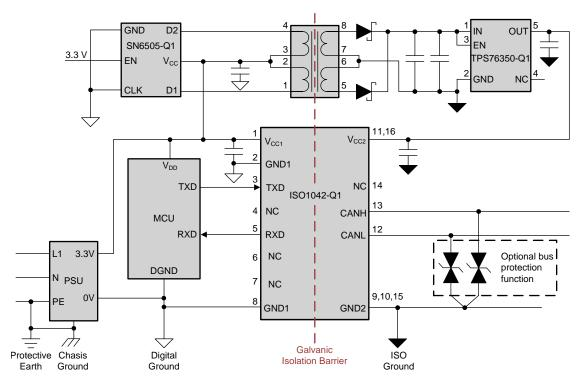
Figure 28. Application Circuit With ISO1042-Q1 in 16-SOIC Package
