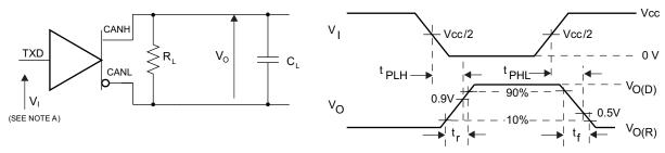
A. The input pulse is supplied by a generator having the following characteristics: PRR  $\leq$  125 kHz, 50% duty cycle,  $t_r \leq$  6 ns,  $t_f \leq$  6 ns,  $t_G =$  50  $\Omega$ .
