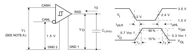
A. The input pulse is supplied by a generator having the following characteristics: PRR  $\leq$  125 kHz, 50% duty cycle,  $t_f \leq 6$  ns,  $t_f \leq 6$
