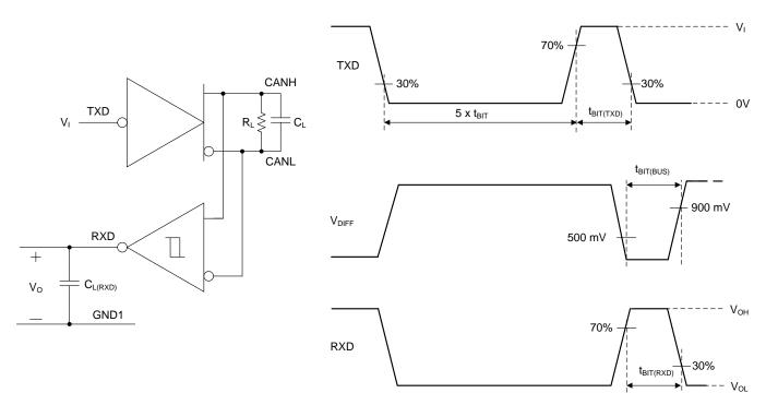
Figure 21. CAN FD Timing Parameter Measurement
