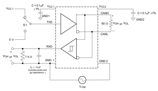
Figure 24. Common-Mode Transient Immunity Test Circuit
