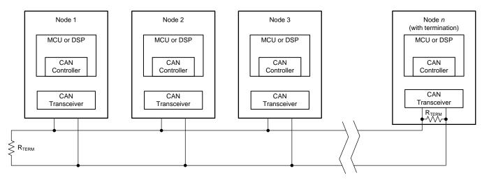
Figure 30. Typical CAN Bus
