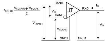
Figure 18. Receiver Voltage and Current Definitions
