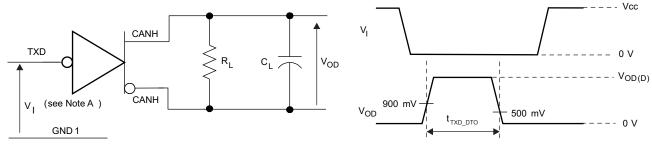
A. The input pulse is supplied by a generator having the following characteristics:  $t_r \le 6$  ns,  $t_f \le 6$  ns,  $t_O = 50$   $\Omega$ .
