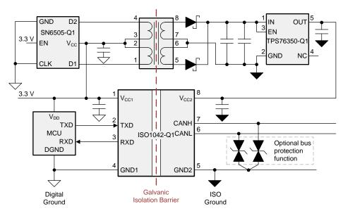
Figure 29. Application Circuit With ISO1042-Q1 in 8-SOIC Package
