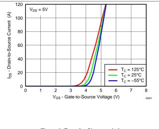
Figure 3. Transfer Characteristics
