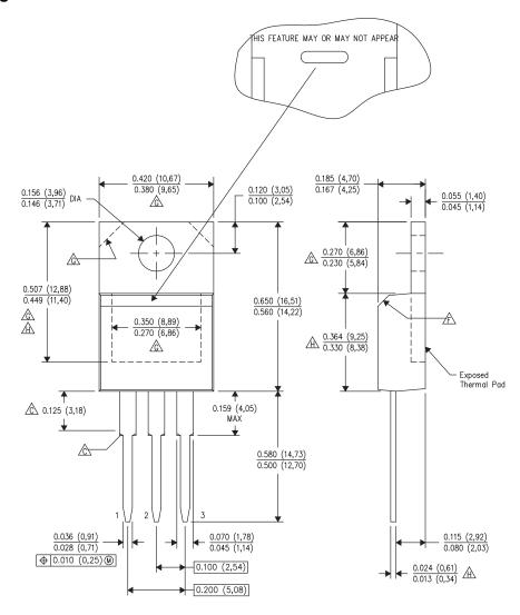
A. All linear dimensions are in inches (millimeters). This drawing is subject to change without notice.
