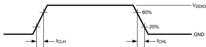
Figure 3. LVCMOS Transition Times
