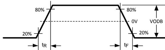
Figure 3. Driver Output Transition Time
