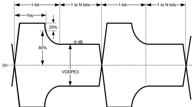
Figure 5. Test condition for output pre-emphasis duration
