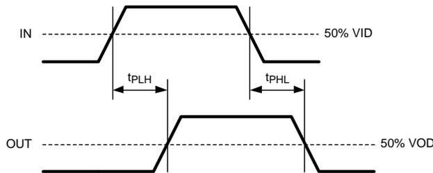
Figure 4. Propagation Delay from input to output
