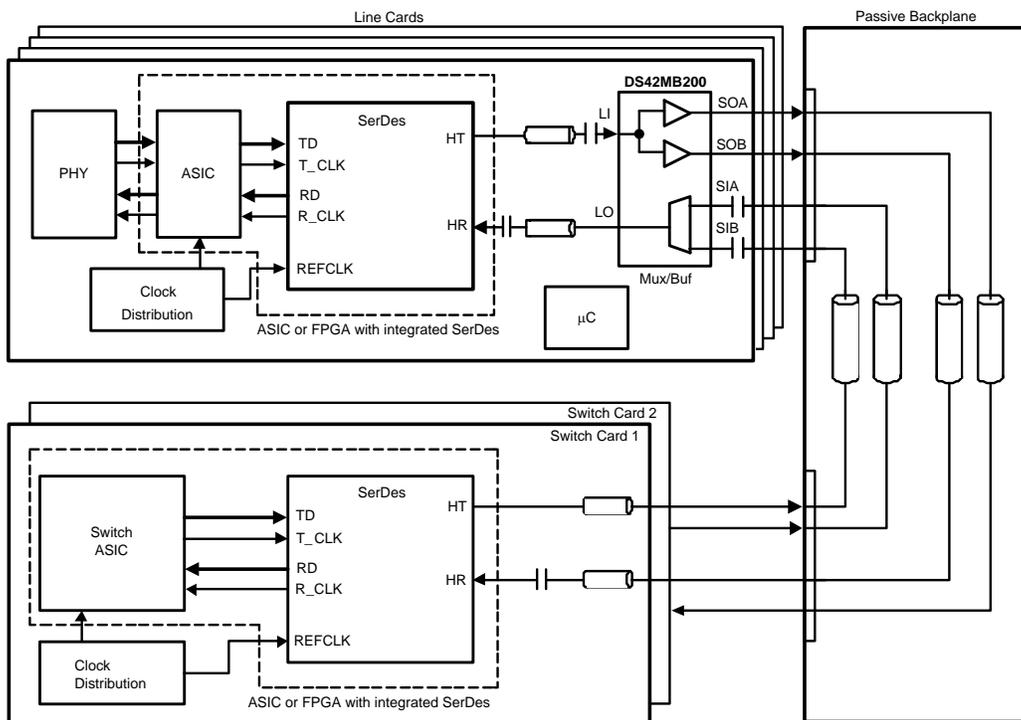
Figure 10. Application diagram (showing data paths of port 0)
