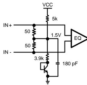
Figure 7. Receiver Input Termination and Biasing Circuit
