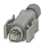
RJ45 connector, Degree of protection: IP67, Number of positions: 8, CAT5 (IEC 11801:2002), Material: PA, Connection method: IDC fast connection, Connection cross section: AWG 26-23, Cable exit: straight
