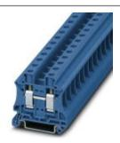
Feed-through terminal block, Connection method: Screw connection, Cross section: 0.5 mm² - 16 mm², AWG: 20 - 6, Width: 10.2 mm, Height: 46.9 mm, Color: blue, Mounting type: NS 35/7,5, NS 35/15
